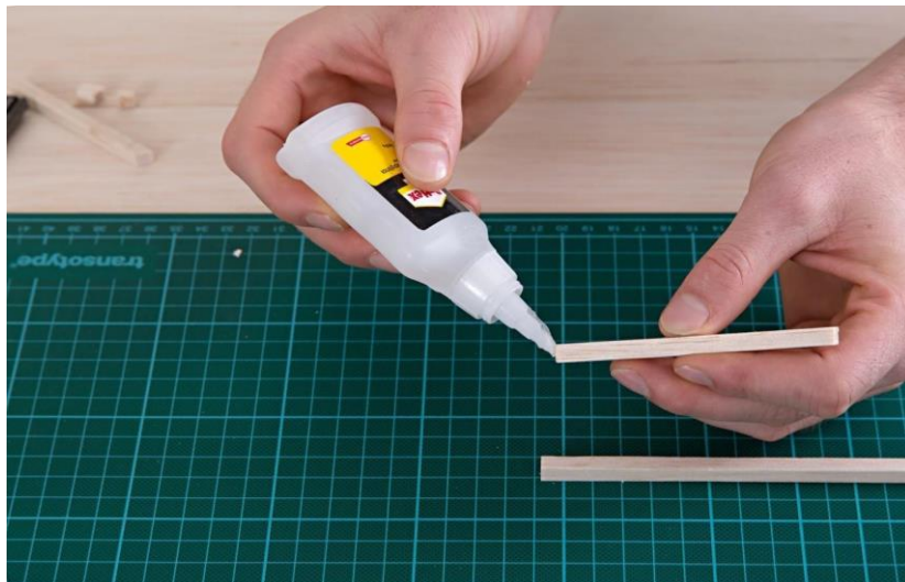
Figure E.5. Gluing of Balsa Sticks
