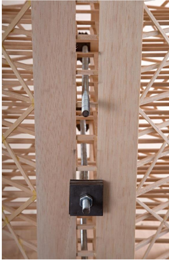
Figure E.14. The Floor Dead Load Rod Must Be Inserted through an Opening between 1.3 cm and 1.6 cm Wide. The Photograph illustrates an incorrect application with an excessively large gap
