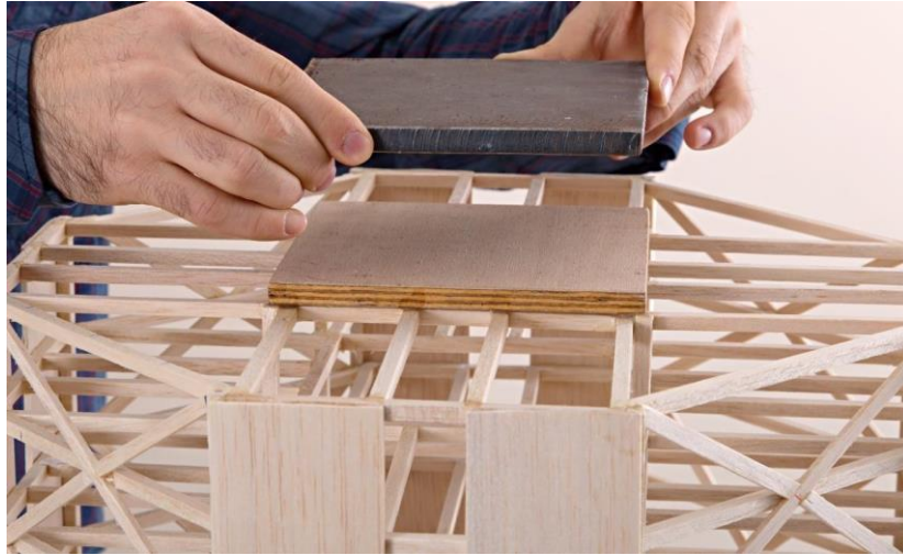
Figure E.12. Metal Plate Glued to Roof Wooden Plate by Teams
